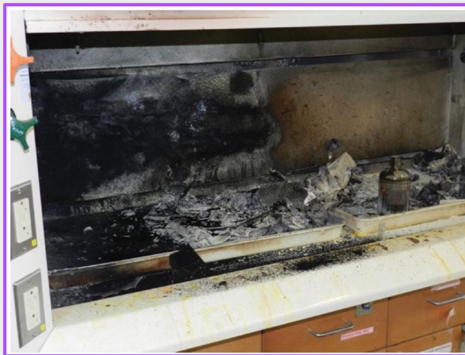
Chemical hood after the explosion due to the rupture of a container from high pressure
